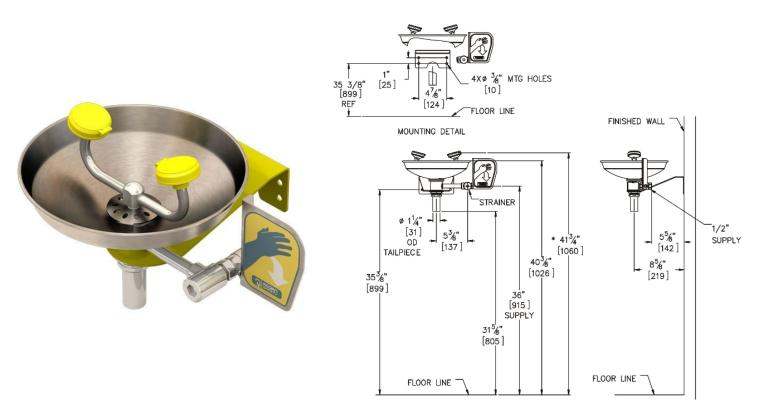
Model S0440 is our wall mounted eye/face wash, with a grade 304 stainless steel bowl, ABS plastic eye/face wash spray heads and dust covers, an inline strainer and a stay-open 1/2" ball valve with a push handle. Comes complete with safety sign and weekly testing card as per ANSI Z358.1 compliance.
